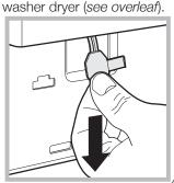
pull outwards using the tab as indicated in the figure, until the plastic tie-rod is freed from its stop position; pull downwards until you hear a "click", which indicates that the door is now unlocked.
